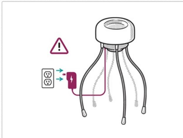
To install the board, you will have to open up Clyde but don't worry, Clyde doesn't bite. Grab Clyde's head, and give it a slight counter-clockwise twist, then gently pull upwards to disengage the top part of the head. It will stay attached by a small wire, and that's fine.
